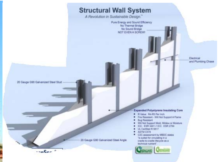
2. Structural Wall System
